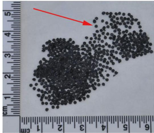
FIG. 8—Photograph of Hornady Custom 9 mm Luger 115 gr. FMJ powder. Zoomed in 50% from original photograph. Arrow indicates disk-shaped powder particle with center perforation. Scale given in cm.
