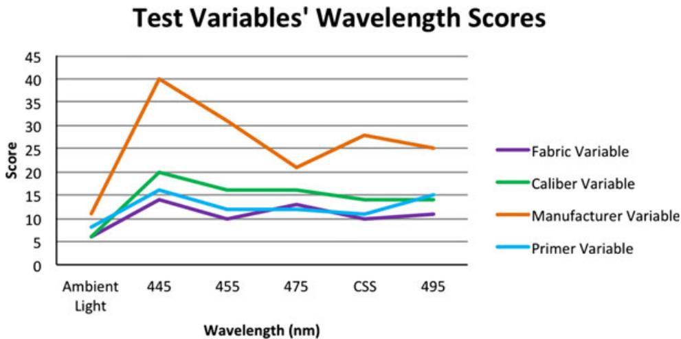
FIG. 5—Shows the average scores of the different variables tested overall (i.e., fabric types and various calibers and manufacturers of ammunition) the wavelength range of main interest. The figure also provides the average scores given to the targets shot with only primed cartridges.
