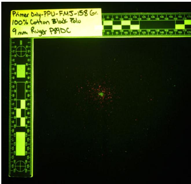
FIG. 3—Photograph of PPU primer residue under 445-nm filter. Scale given in mm.
