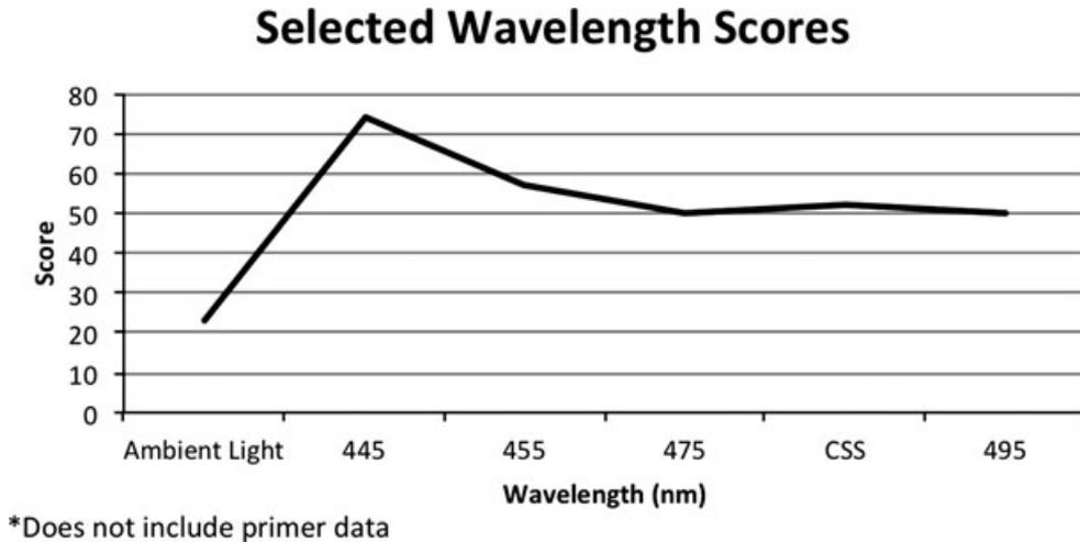
FIG. 4—The total scores for all targets analyzed using the 445-nm to 495-nm filters, as compared to ambient light. The same criterion as described in Fig. 1 was used to assign scores.
