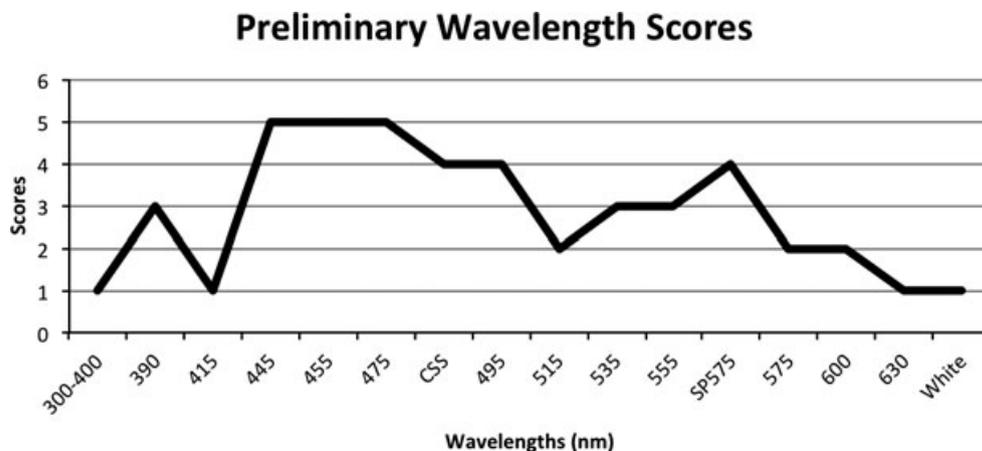
FIG. 1—Values ranging from one to five given for the performance of the 16 wavelengths tested on the Mini-CrimeScope. The lowest score of one meant no particles could be seen, or there was poor contrast between particles and the background. The highest score of five was assigned to those with great contrast and little to no loss in visualization of particles.
