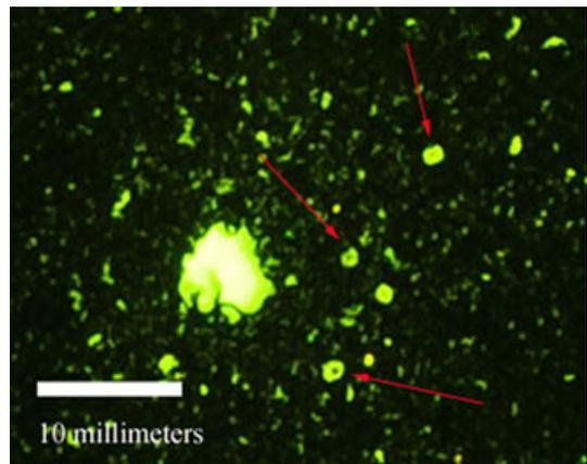
FIG. 9—Photograph of Hornady residue under 445-nm filter. Zoomed in 200% from original photograph. Arrows indicate intact, unburnt gunpowder residue displaying center perforation characteristic, as shown in Fig. 8. Scale bar indicates 10 mm.
